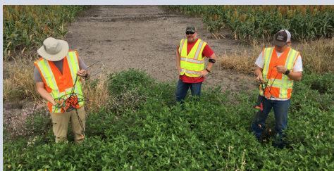
KCC staff members Jonathan Hill, David Bollenback and Jake Eastes prepare geophones for use at the Knackstedt remediation site in McPherson County. Geophones are placed on the ground and used to detect seismic waves. The Knackstedt Site involves an unplugged saltwater disposal well with severe casing failure, causing dissolution in the Hutchinson Salt section, leaving an air filled void around the well. The seismic survey will help define the extents of the void, and depths where dissolution has taken place.
