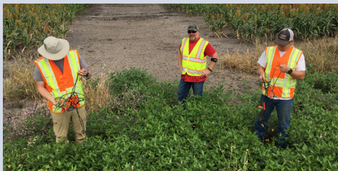
KCC staff members Jonathan Hill, David Bollenback and Jake Eastes prepare geophones for use at the Knackstedt remediation site in McPherson County. Geophones are placed on the ground and used to detect seismic waves. The Knackstedt Site involves an unplugged saltwater disposal well with severe casing failure, causing dissolution in the Hutchinson Salt section, leaving an air filled void around the well. The seismic survey will help define the extents of the void, and depths where dissolution has taken place.
