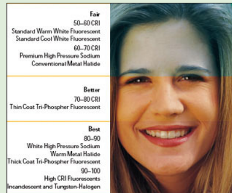
Figure 4: As CRI decreases, the accuracy of the color decreases.
